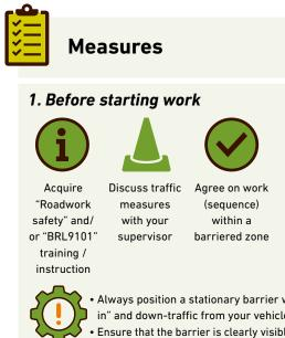
• Always position a stationary barrier working "outside in" and down-traffic from your vehicle. • Ensure that the barrier is clearly visible to road users
